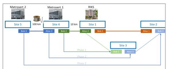
In the second phase, the third QKD device pair will be introduced to the round network, and a comprehensive circular solution will undergo initial testing, starting with lower speeds on 10G ports. During this phase, rigorous operational, management, and monitoring tests will be conducted. This stage is crucial to ensure the stability of both the QKD and network devices, guaranteeing their reliable integration and operation before implementing the technology for high-speed connections.
